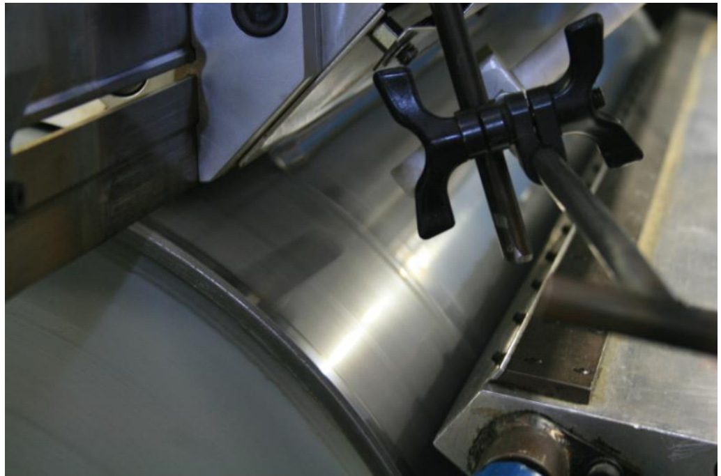
Molten plastic hits the chill roll on a cast extruder, dropping 445°F within 1/10th of a second.
